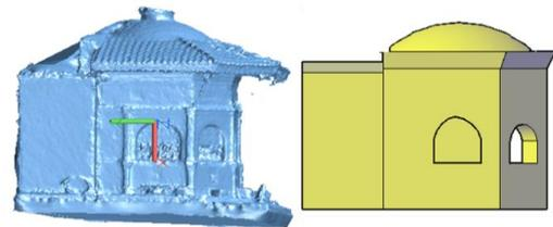
Figure 4: Left: Agisoft's mesh Right: Solid model.
